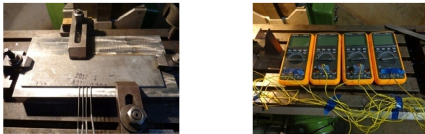
Fig. 2. (a) Close view of experimental setup, (b) Close view of four multimeters connected to thermocouples.
