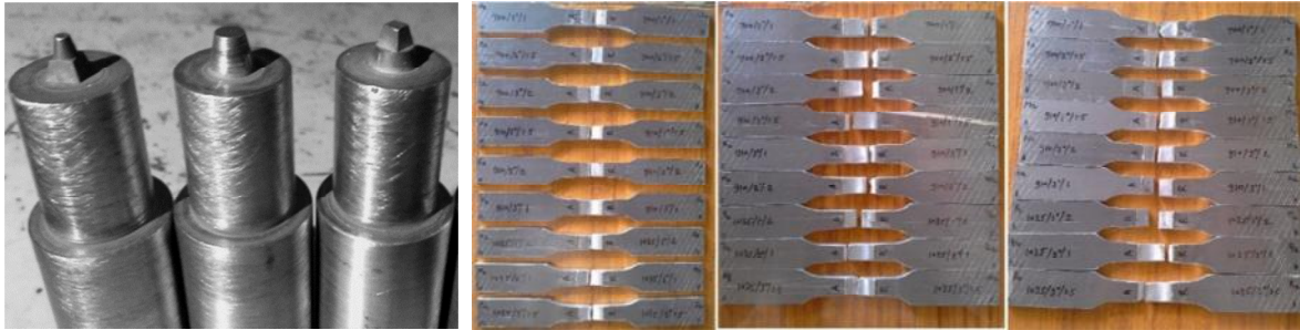
Fig. 2. (a) Friction Stir welding tools; (b) FSW tensile strength tested samples.
