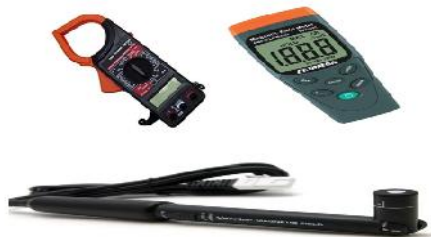
Fig. 2: Advanced meters/ sensors for Magnetic field measurement
