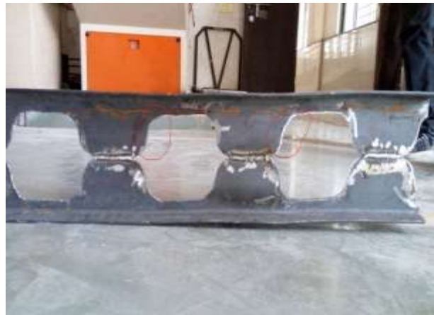
Figure 3 Shear Stress Redistribution In I S1
