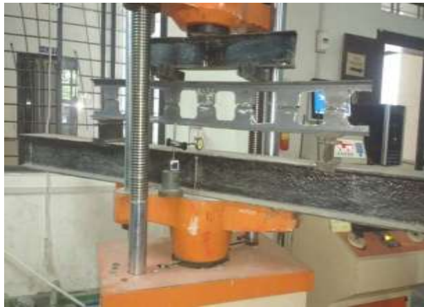
Figure 2 Testing Arrangement of Castellated Beams
