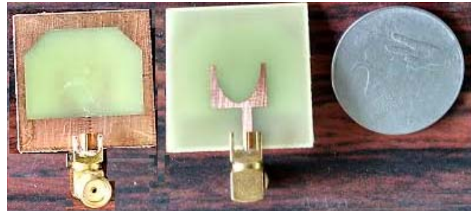
Fig 2.Prototype of fabricated antenna
