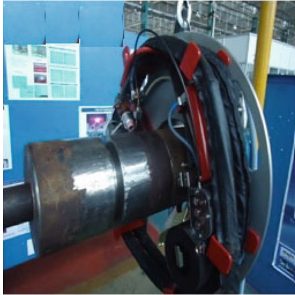
Fig. 6 Orbital hotwire GTAW (Santhakumari 2018)
