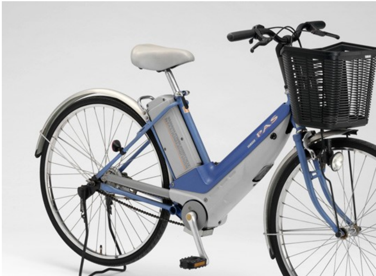
Fig.23. An illustration of a electrically power-assisted bicycle( pedelec) [38].
