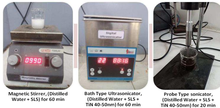
Figure 2. Preparation of Stable TiN Nanofluid
