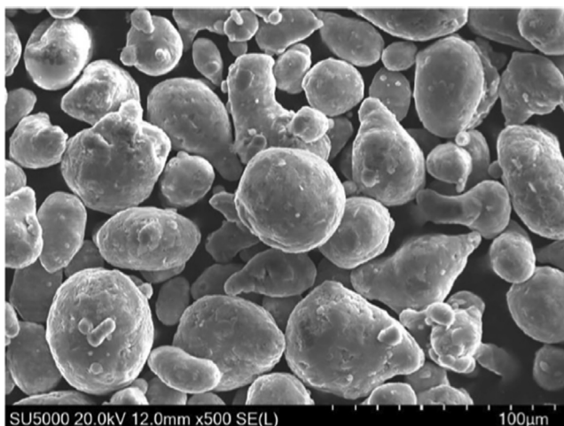
Fig. 1. Morphology of gas atomized AlSi10Mg alloy powder [27].
