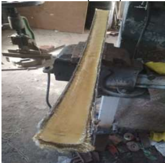
Fig (3.1): Composite laminate specimen prepared in laboratory by hand lay up method.
